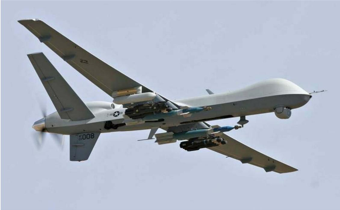
BALAD AIR BASE, Iraq (AP) The airplane is the size of a jet fighter, powered by a turboprop engine, able to fly at 300 mph and reach 50,000 feet. It is outfitted with infrared, laser and radar targeting, and with a ton and a half of guided bombs and missiles.
